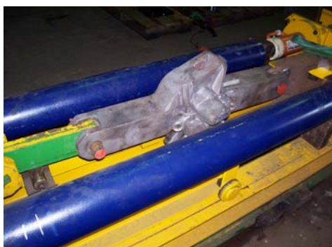
Proof load of a Willison Coupling
