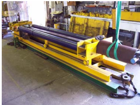
Proof load of an Extended Drawbar
