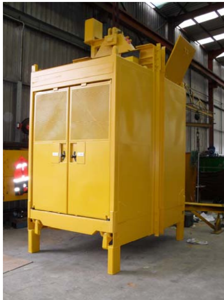
Man Cage for vertical shaft
